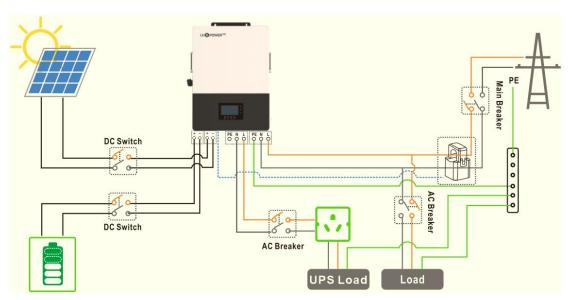
Hybrid inverter will not only provide power to the backup load connected but also give power to the home load connected. If PV power and battery power is insufficient, it will take grid energy as supplement. The hybrid inverter will not sell power to grid. The external CT(&Meter) will detect power flowing back to the grid and will reduce the power of the inverter only to supply the local load, charge battery and home load. This control is achieved by:
