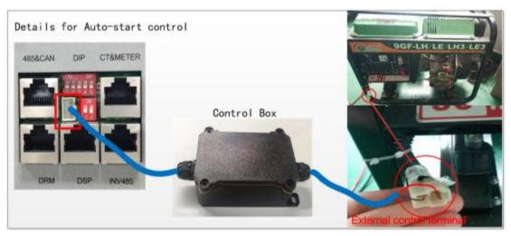
Notice: 1. The Generator itself should support auto-start function which may be named as "remote start" and physical terminal might be the "AUX input" and the "GND" (Read the manual of generator carefully)
