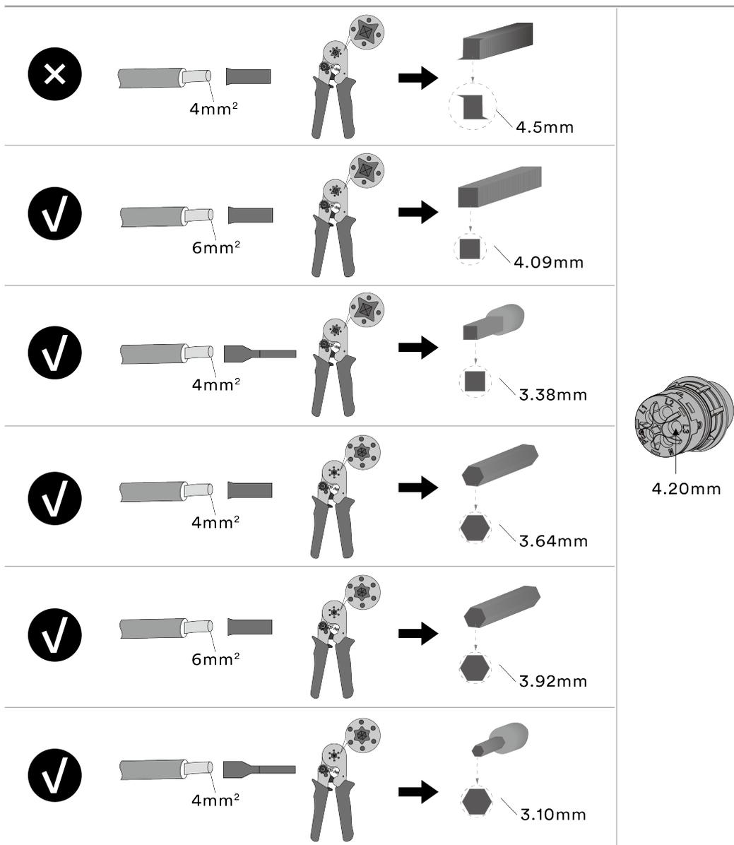
**Step 4:** Set the parts on the cable, insert the terminal holes in sequence. Crimp the wire with an inner hexagon screwdriver and screw the torque 1.2+/-0.1N·m.
