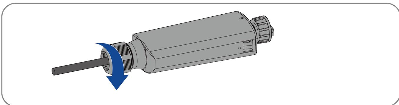
**Step 4:** Remove the dust and waterproof cover of the INV Logger V200 on the inverter and retain it.
