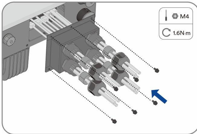
**Step 5:** Tighten the cable gland nuts.
