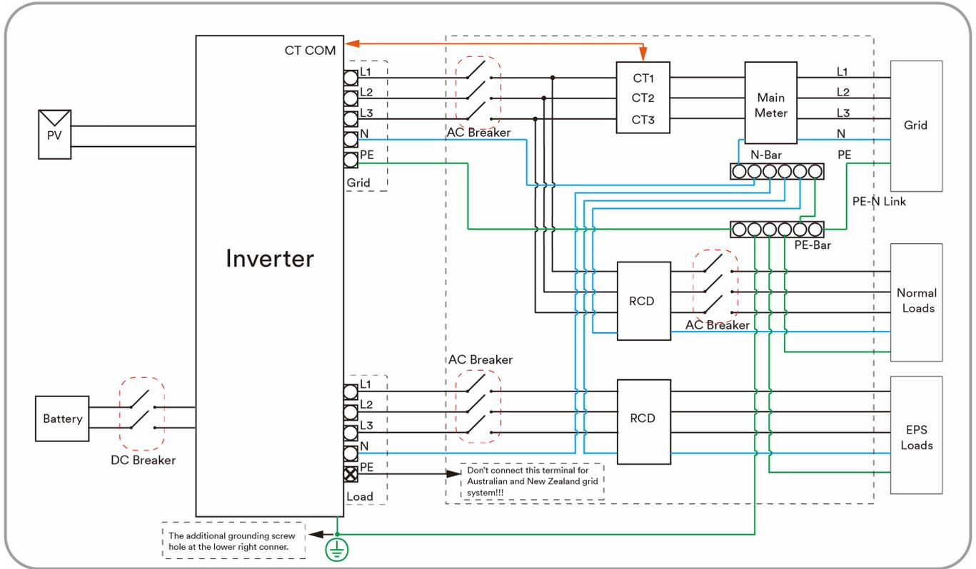
For other countries, the following diagram is an example for grid systems without special requirement on wiring connection.
