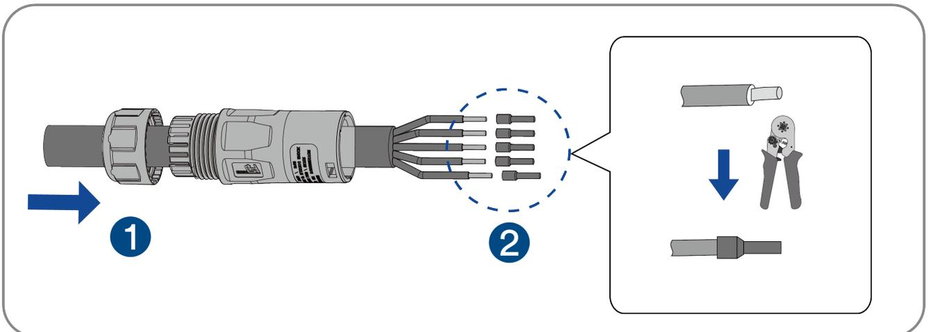
Crimping tool selection and crimping requirements are shown in the following figure:
