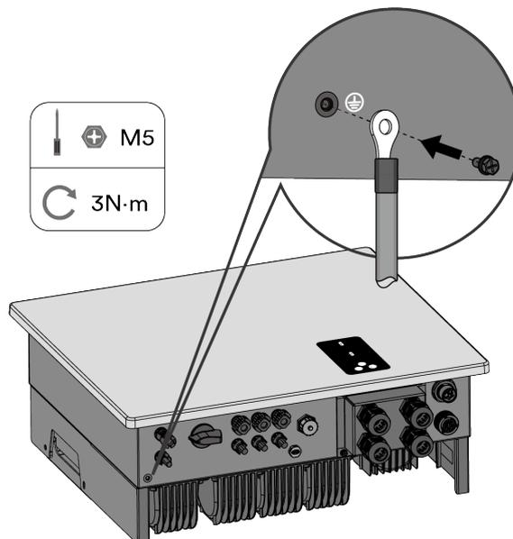
**Step 3:** Apply paint to the grounding terminal to ensure corrosion resistance.
