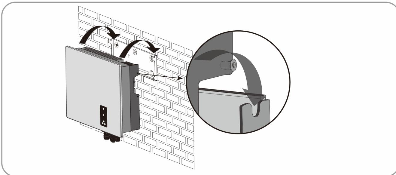
**Step 5:** Fix the inverter with screws.
