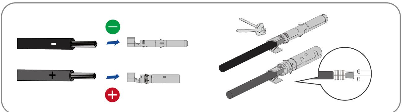
**Step 3:** Lead the cable through cable gland, and insert into the insulator until it snaps into place. Gently pull the cable backward to ensure firm connection. Tighten the cable gland and the insulator (Torque 4Nm).
