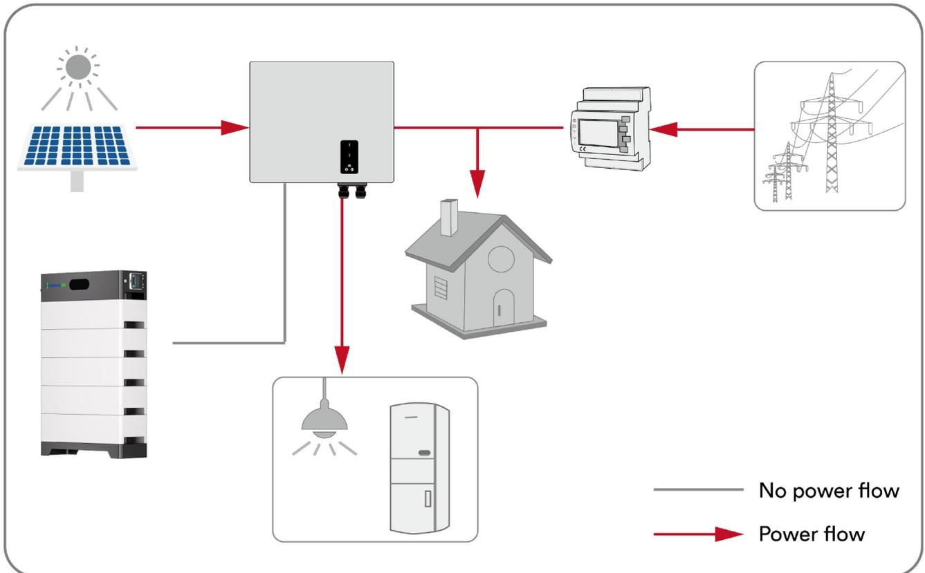
Case 2: PV power generation is lower than the load power consumption, and the energy of the battery is available.
