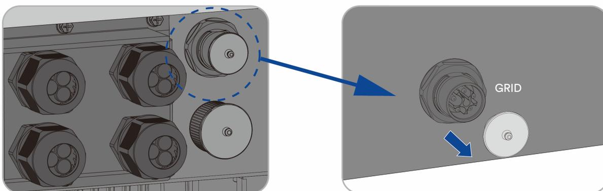
**Step 2:** The installation arrow indicates insertion the female connector, and hear the “click” sound.
