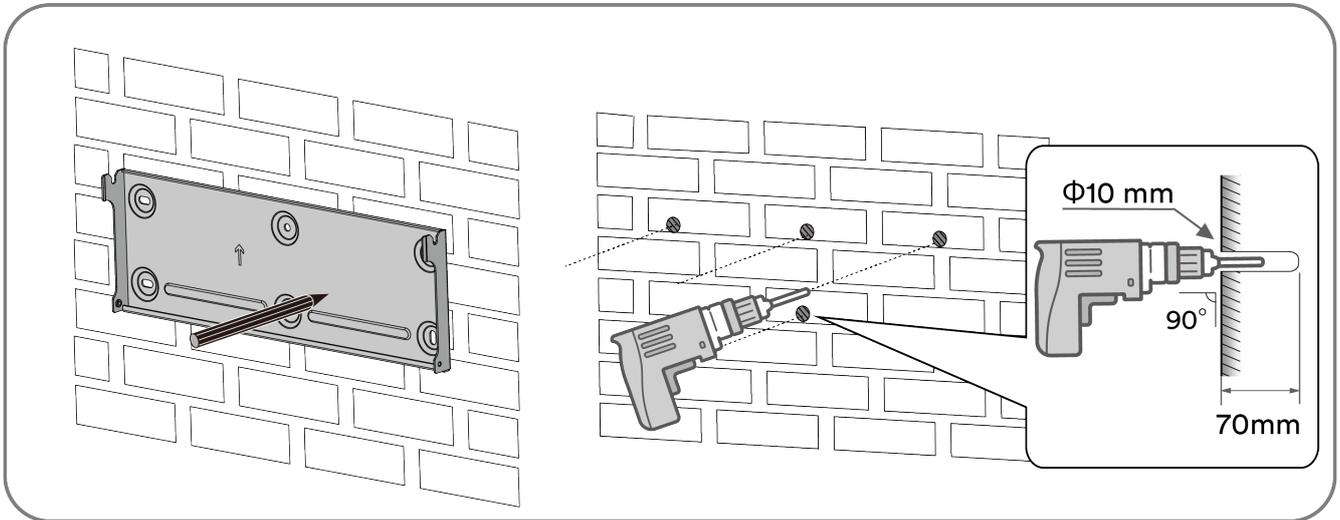
**Step 2:** Hammer the plastic expansion pipe slowly into the drilled hole.
