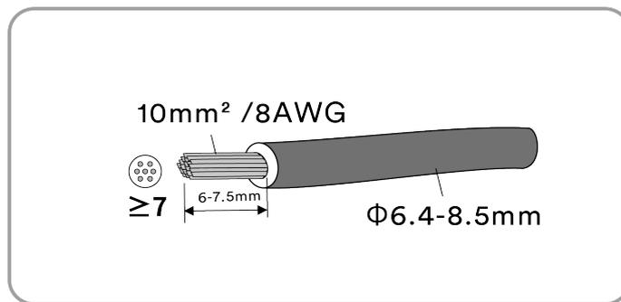
**Step 2:** Assemble the cable ends with the crimping pliers.
