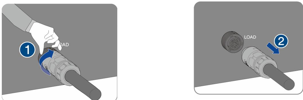
**Step 9:** Loosen and remove the Battery connector.
