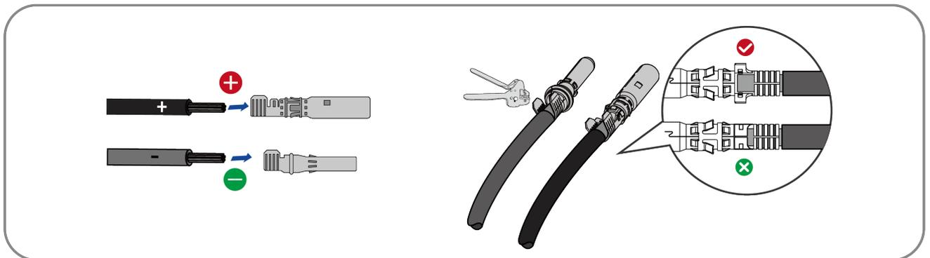
**Step 3:** Lead the cable through cable gland, and insert into the insulator until it snaps into place. Gently pull the cable backward to ensure firm connection. Tighten the cable gland and the insulator (Torque 2.5-3Nm).
