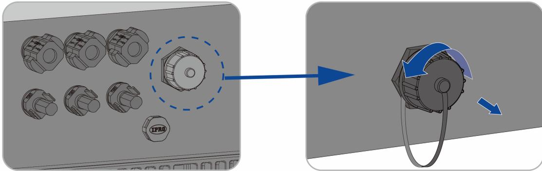
**Step 5:** Attach the INV Logger V200 to the connection port in place and tighten it into the port by hand with the nut in the modular. Make sure the modular is securely connected and the label on the modular can be seen.
