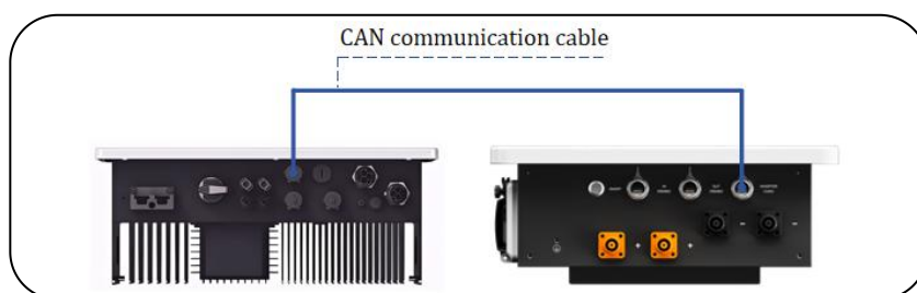
Figure 18 Sample of Connecting the CAN Communication Cable
