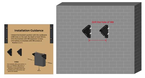
2. Tighten the screws between the bracket and the battery with 2.5N.m torque.Two or four batteries can be installed by these brackets.
