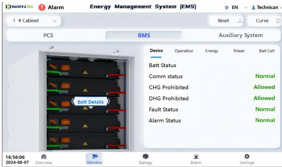
Figure 7-9 Detail information of battery cell
